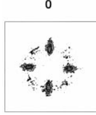
Fig. 3. The diffraction pattern when B , c and the neutron beam are aligned (0.5 T, 5 K, sample II).
